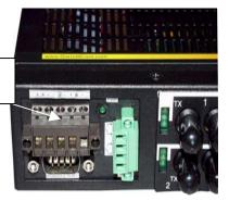
Figure C5.0: -48VDC Dual-Source, wiring connections to the External Terminal Block on a Magnum -48VDC with Dual-Source option
